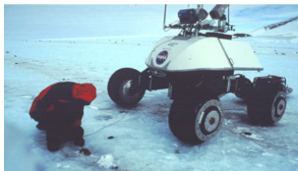
Figure 2: Human assisted rock/meteorite classification during the second Antarctic expedition at Patriot Hills in November 1998. Human deploys the spectrometer, then the robot analyzes the data.
