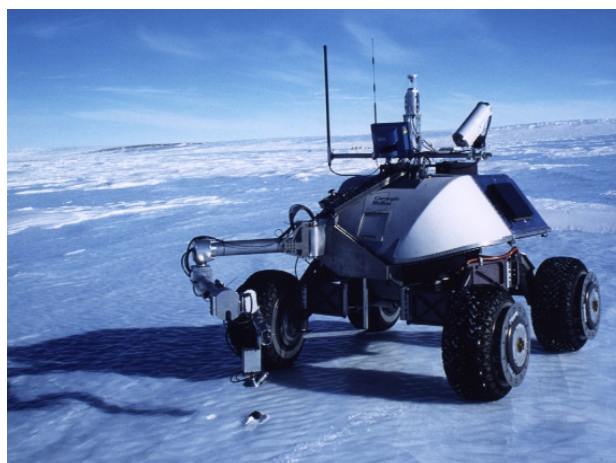
Figure 3: Nomad autonomously investigates a meteorite sample using its manipulator arm at Elephant Moraine, Antarctica, in January 2000.
