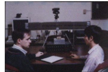
Figure 9. Setup of microphone array and face tracker
