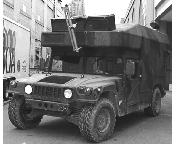
Fig. 7 The autonomous vehicle (HMMWV) that used for our experiments. The vehicle is equipped with stereo vision, inertial guidance and GPS positioning.
