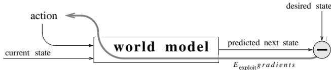
Figure 2: Using the model for optimizing actions (exploitation). Starting with some initial action, gradient descent through the model network progressively improves actions.
