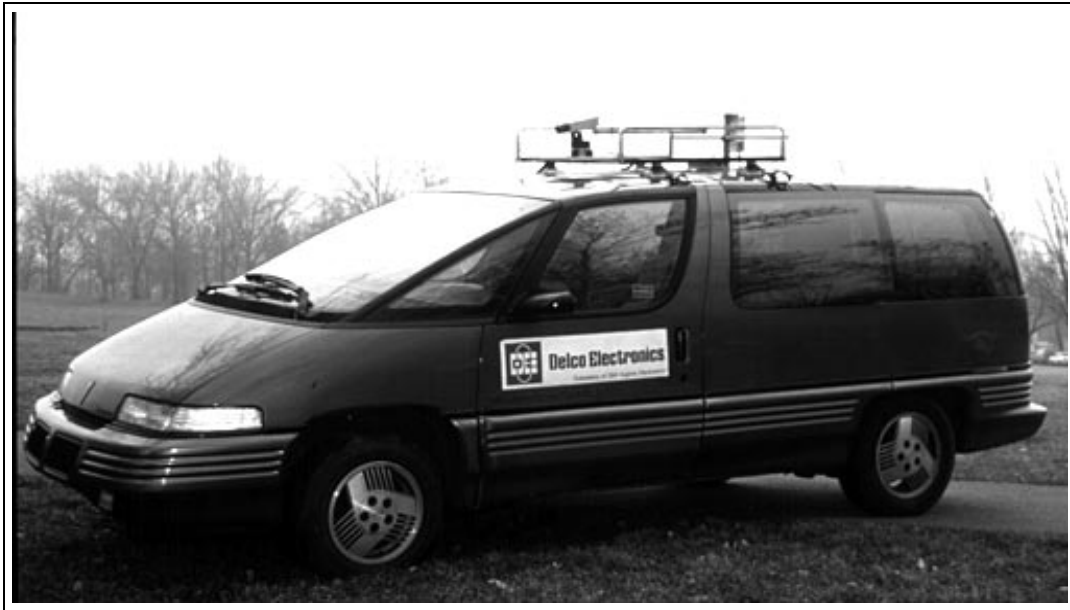
Figure 5: The Carnegie Mellon Navlab 5 is a testbed for developing autonomous navigation systems. Wherever possible, SHIVA is compatible with existing perception and control modules available on the Navlab.
