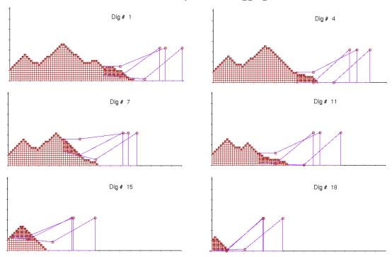
Figure 9. Simulated progression of a loading task.
