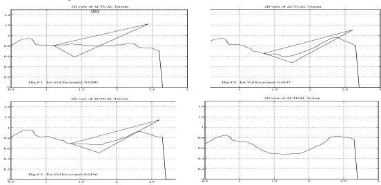
Figure 11. Progression of terrain during trenching task.
