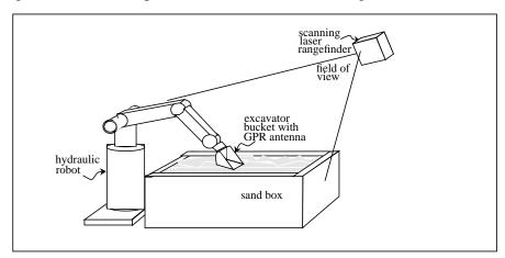
Figure 10. Excavation testbed
