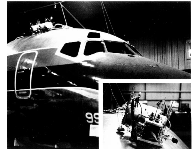
Fig. 2: Photograph of ANDI on nose of DC-9 at Aging Aircraft Nondestructive Testing Center.
