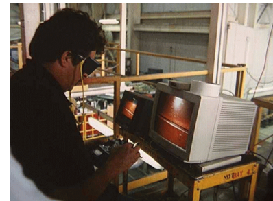
Fig. 5: Aircraft inspector observing the live stereoscopic imagery on the video monitor using active eyewear
