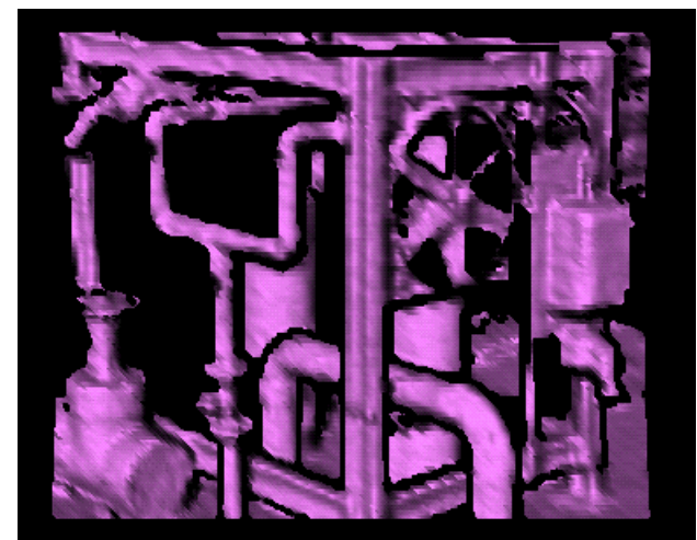
Figure 5. Shaded views of a scene surface mesh before (top) and after (bottom) processing. Processing removes pixels on range discontinuities, removes small patches and low-pass filters the data.
