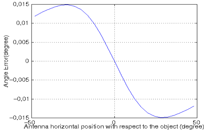
Figure 47. The error in the reflection angle computation using the flat reflector method for a point reflector.
