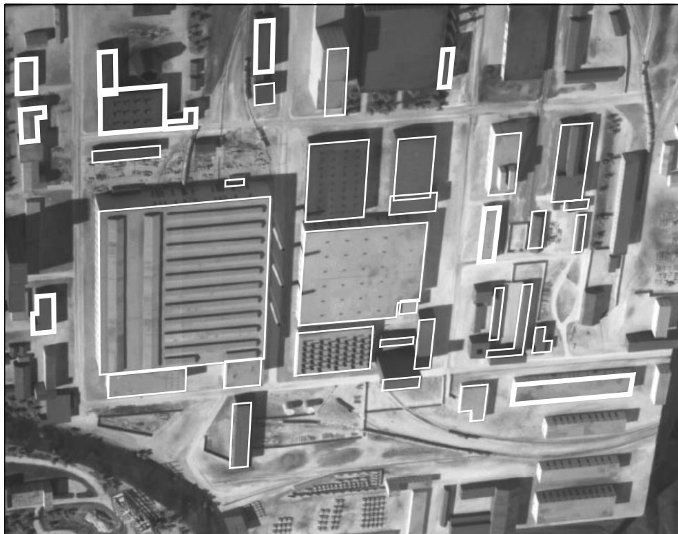
Figure 12. Updated site model projected onto image J8. Thin lines denote the registered partial site model. Thick lines delineate buildings that were automatically detected and added via model extension.
