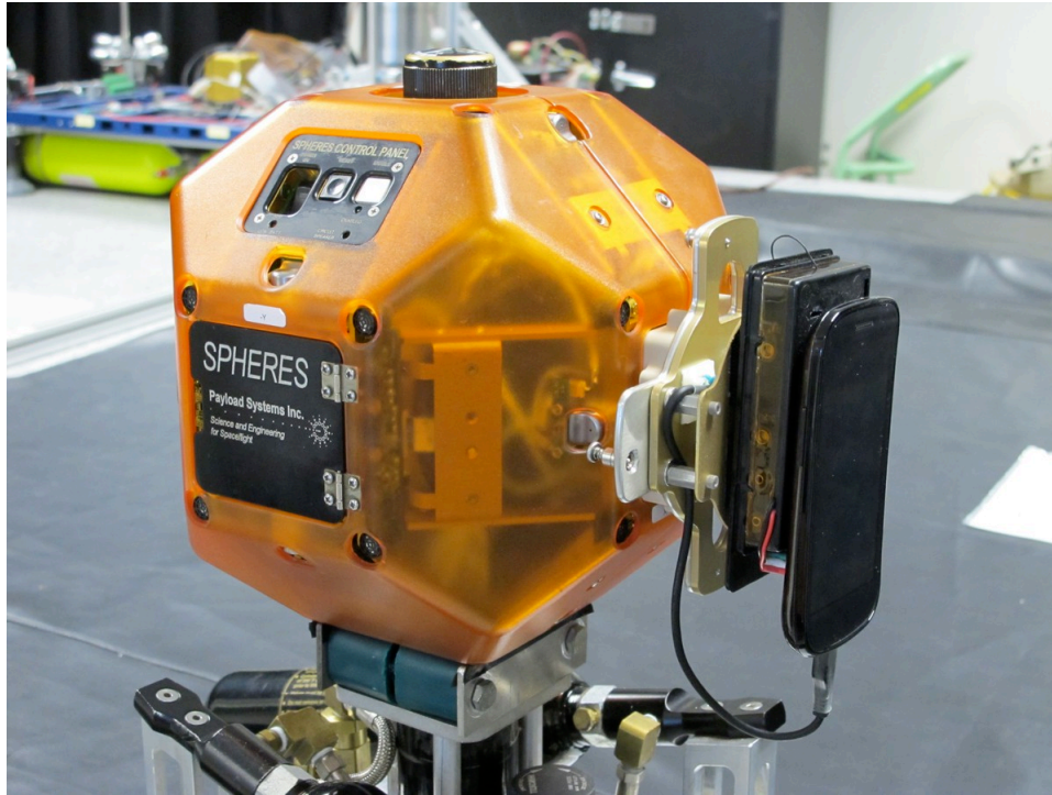
Figure 2. Smart SPHERES combines a modified Android smartphone with SPHERES. The smartphone is attached to SPHERES via the expansion port. This image shows the robot in a laboratory at NASA Ames, where it is tested using an air carriage on a granite table.
