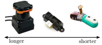
Figure 1.6: Different sensing modalities have different maximum ranges. LIDAR (left) has a long range, near-touch sensors (middle) have a short range, and contact sensors (right) have zero range.
