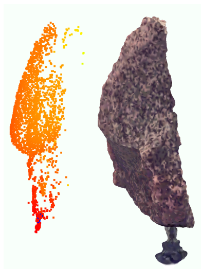
Figure A.20: Comparing a reconstructed point cloud to the coarse mesh model. Points in the reconstructed cloud are colored by distance from the mesh.
