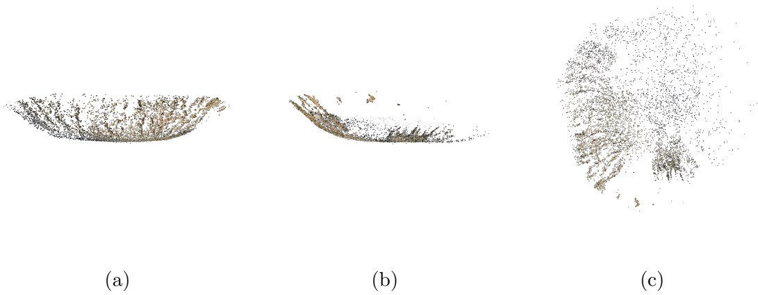
Figure 6.39: Sparse reconstruction of meteor crater: (a) side view, (b) view from behind the camera, (c) top view
