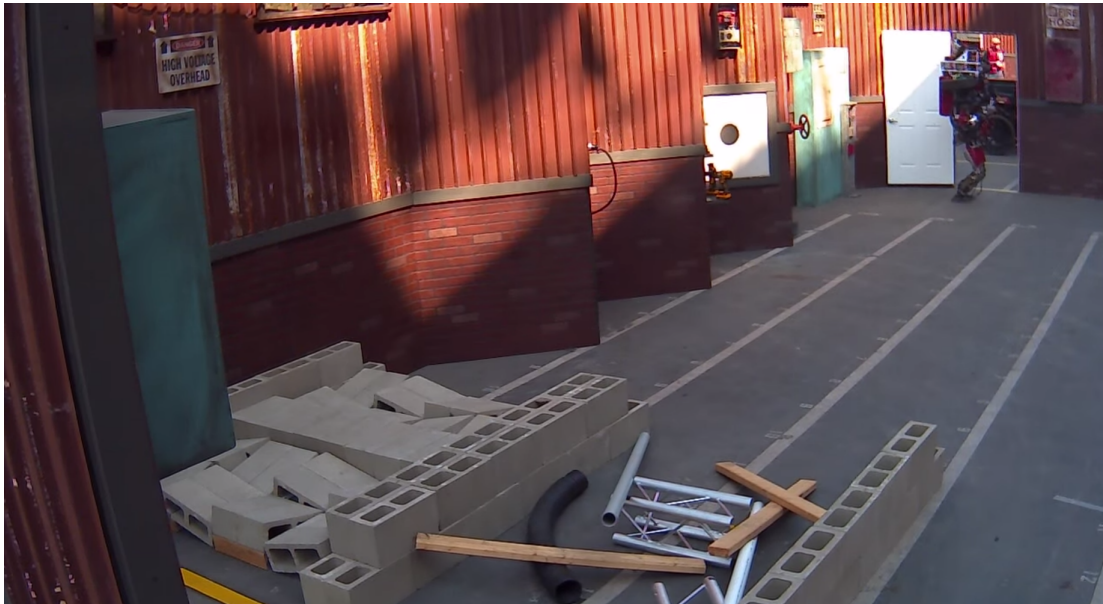
Figure 3.9: Picture taken from the second run of team WPI-CMU in the DRC Finals, showing part of the course setup. At the bottom of the picture is the rough terrain, in the middle is the manipulation tasks setup, and on the top right corner is the Atlas robot passing through the door.
