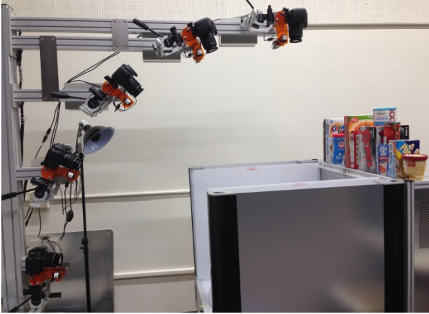
Fig. 8: BigBIRD Object Scanning Rig: the box contains a computer-controlled turntable.
