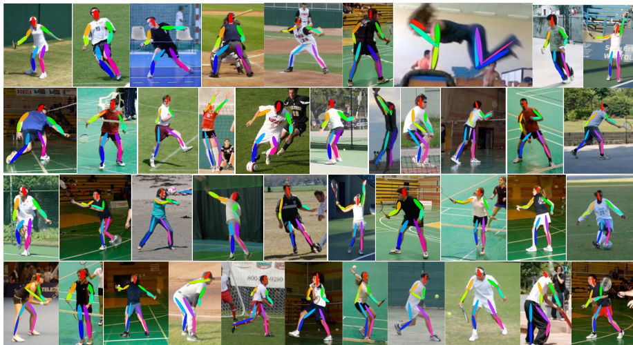
Fig. 7: Qualitative example results on the LEEDS sports dataset. Our algorithm is able to automatically learn a spatial model and correctly localize traditionally difficult parts such as the elbows and wrists.
