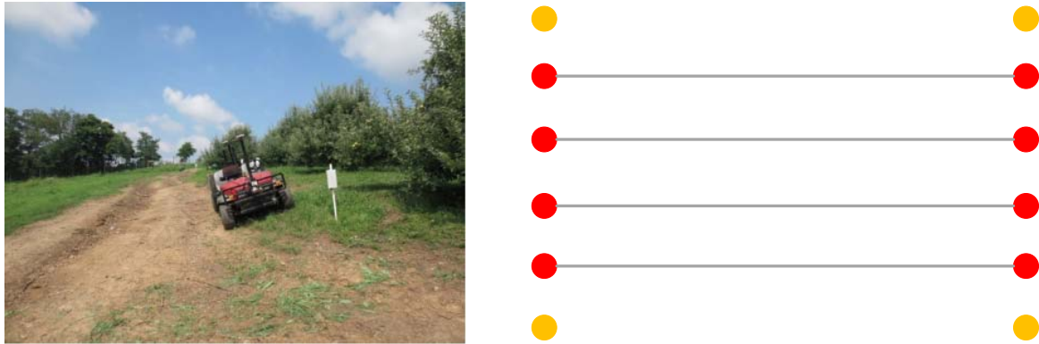
Figure 7. Left: Example of steep headland that causes significant wheel slip and where the normal mapping method fails. In these situations we install four additional landmarks, represented by the yellow circles on the right, that introduce four new geometric constraints to the mapping process. The additional landmarks have extended the range of blocks that can be mapped and therefore the range of blocks in which the autonomous orchard vehicle can operate.
