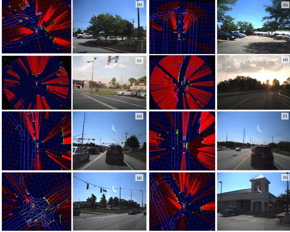
Figure 6: Examples of the resulting instantaneous, omni-directional views of obstacles around our self-driving car. Some objects appeared on these views not appeared on the image of the same scene. This is because a LIDAR’s horizontal FOV (e.g., 100^\circ ) is wider than that of our camera (e.g., 58^\circ ). The resolutions of the map views vary because we zoomed in (or zoomed out) based on the interesting parts of the scenes.
