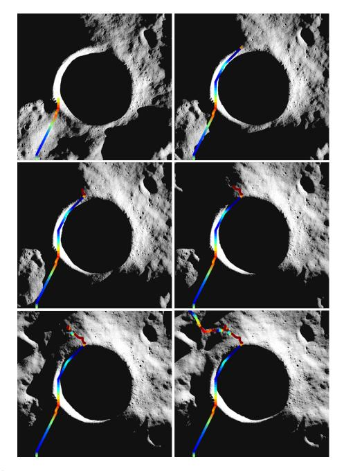
**Figure 3.** A simulated traverse around Shackleton Crater on the Moon demonstrating the planner's ability to plan through time in a dynamic environment. Successive images represent evenly spaced snapshots in time of the rover's path. The path is colored by the amount of energy the rover has. Blue and red correspond to the minimum and maximum energy levels, respectively.
