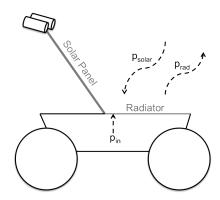
Figure 2. Diagram of heat flow
