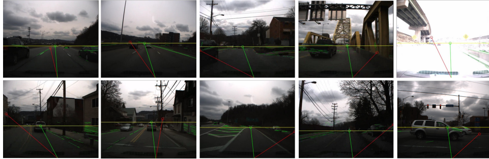
Figure 4: A comparison of vanishing point locations by the frame-by-frame detection and by the EKF tracking.
