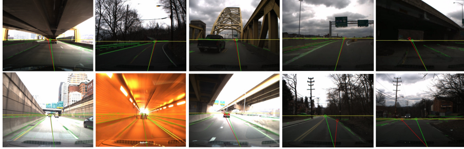
Figure 3: Some examples of vanishing point detection results. For most of testing images, our vanishing point detection worked well as good as tracking method. But it often failed to correctly identify the location of the horizontal vanishing point. For the last two images, our detection method found the locally optimal vanishing points (red circles) based on the lines extracted from those images. By contrast, our tracking method were able to find the globally optimal locations (green circles) of the vanishing points.
