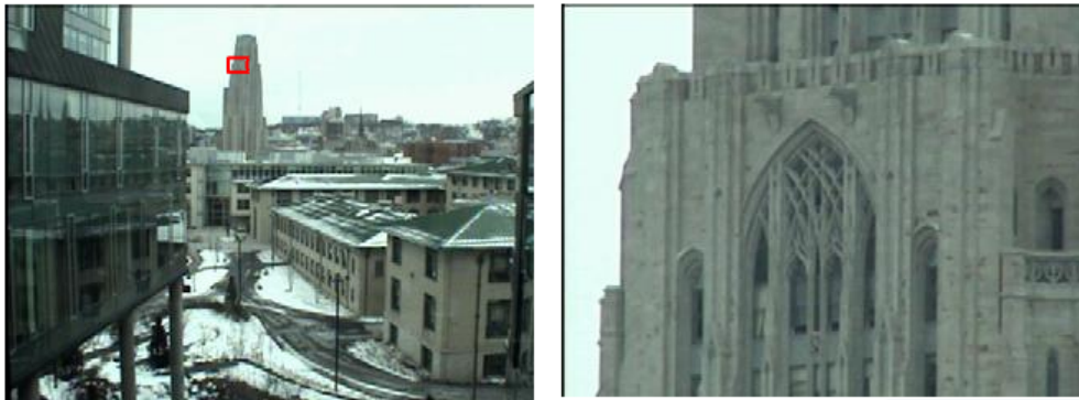
Figure 3.9: At left, CoBot-2 views a scene at the default zoom level. At right, the user zooms in to the boxed area at the maximum level of 18X. The powerful zoom functionality of the robot allows users to inspect small or distant objects, and even read text remotely. Only CoBot-2 possesses such a powerful camera.
