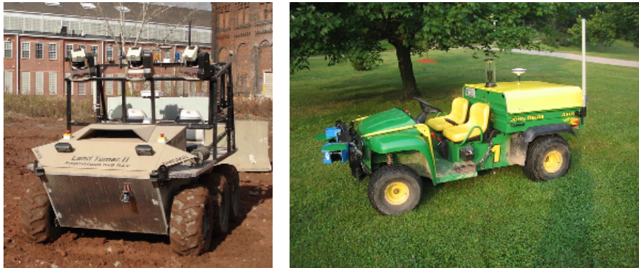
Figure 3.12: (Left) Photograph of the LandTamer, a six-wheeled skid-steer vehicle made by PFM Manufacturing Inc. (Right) Photograph of the RecBot, a John Deere Gator retrofitted for unmanned operation. The RecBot is fully electric and Ackerman-steered.
