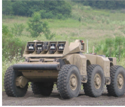
Figure 3.2: A Photograph of the Crusher vehicle, built by the National Robotics Engineering Center (NREC) with support from DARPA.
