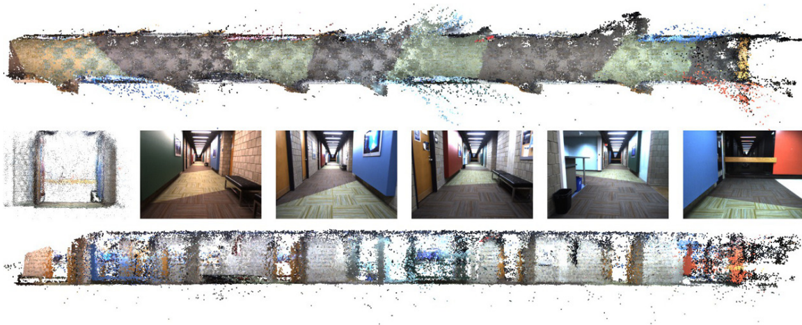
Figure 19: First row shows a top view from our indoor dataset. Images along the corridor are shown in the second row. The first image shows that floor of the model is flat as expected. The last row shows a side view of the corridor. The 3D points are obtained automatically from the algorithm without post-processing or filtering. The corridor length is \approx 40 m.
