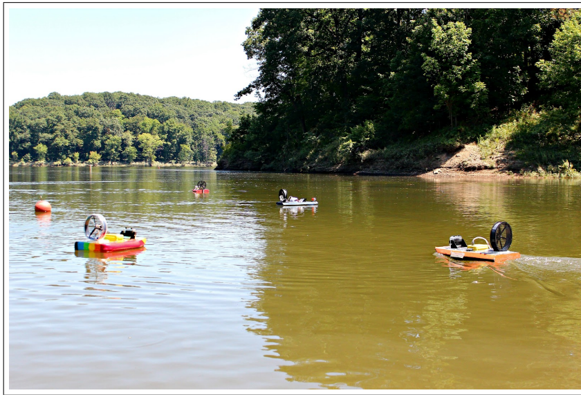
Fig. 1. Multiple watercraft robots autonomously monitoring oxygen and temperature levels in a riverine environment
