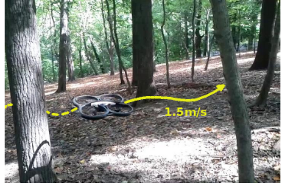
Fig. 1. We present a novel method for high-speed, autonomous MAV flight through dense forest areas. The system is based on purely visual input and imitates human reactive control.
