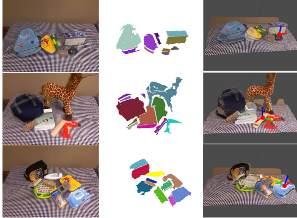
Fig. 4: Experimental evaluation of facet detection. Left: pile of unknown objects. Middle: segmentation of the scene into facets (color coded). Right: 3D view of the scene. To interact with objects we instantiate compliant controllers with information extracted from each facet: COG (red circle) and principal axes (red = principal axis, green = secondary axis, blue = trinary axis).
