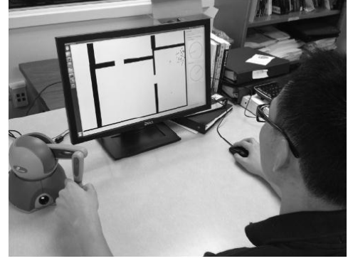
Figure 2 Participants used an Omni Phantom device and mouse to influence the swarm and manipulate the interface respectively.
