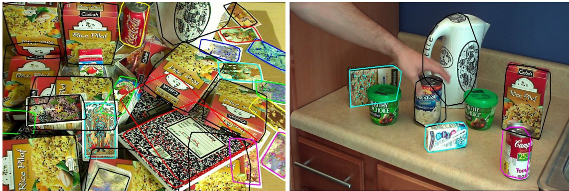
Figure 2.3: Recognition of real-world scenes. (Left) High-complexity scene. MOPED finds 27 objects, including partially-occluded, repeated and non-planar objects. Using a database of 91 models and an image resolution of 1600 \times 1200 , MOPED processes this image in 2.1 seconds. (Right) Medium complexity scene. MOPED processes this 640 \times 360 image in 187 ms and finds all known objects (The undetected green soup can is not in the database).
