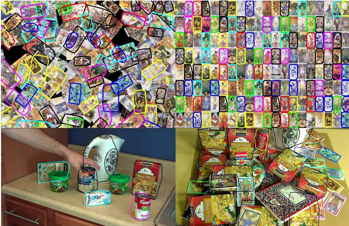
Figure 4.4: MOPED Benchmarks. For the sake of clarity, only half of the detected objects are marked. (a) The Rotation Benchmark: MOPED processes this scene 36.4x faster than the Baseline. (b) The Zoom Benchmark: MOPED processes this scene 23.4x faster than the Baseline. (c) The Simple Movie Benchmark. (d) The Complex Movie Benchmark.
