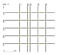
Figure 2: A 5X5 grid network of 25 intersections
