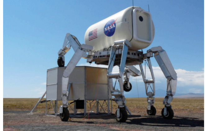
Figure 1. The “T12” ATHLETE robot stepping off of a simulated lander.
