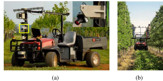
Fig. 1. (a) The robot. A monocular camera is attached in front of the robot as highlighted by the yellow box, a closed view of the camera is shown in the small thumbnail at the right-top corner. (b) The robot drives autonomously along the tree rows. In this example, a liftable platform is attached on the back of the robot, the platform carries two workers.
