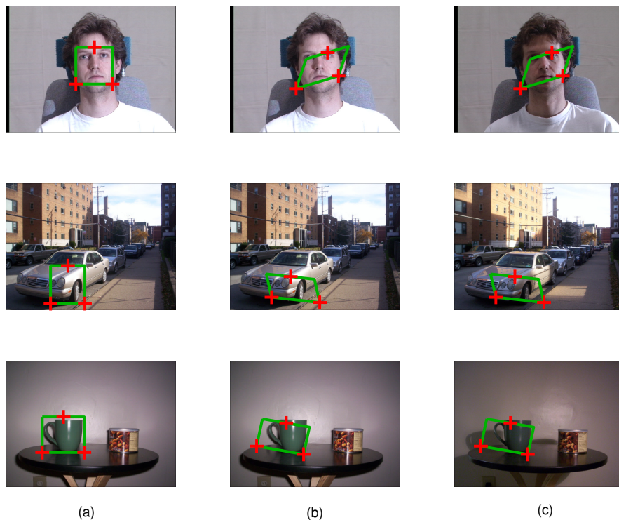
Fig. 1. (a) A template centered around the object of interest with three canonical points shown as red pluses. (b) Sample warps defined by the random perturbation of the three canonical points. (c) Sample warps shown on an image that has different illumination conditions as compared to that of the template for various objects.
