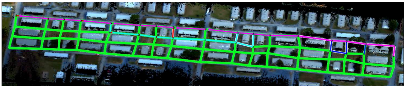
Figure 5.10: New paths are replanned for the updated graph. These four paths start at the vertices where the previous traversals ended.
