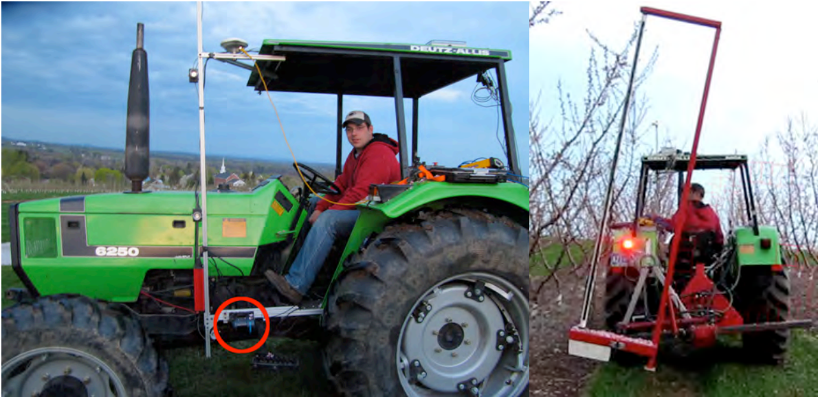
Figure 4: Picture of the system used from side (left) and rear (right) views. Note the laser scanner in the bottom center of the side view (surrounded by red)– it scans in a plane parallel to the thinning plane.
