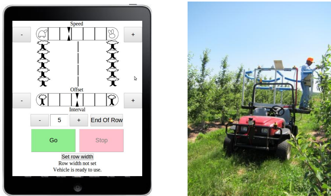
Figure 8. (Left) Grower-friendly interfaces are an important element of the overall usability aspect of autonomous vehicles. Our current interface, based on formal human-computer interaction methodology, runs through a web browser on any mobile device. It allows workers to control the desired speed and lateral position of the vehicle in the row, and also provides workers with feedback on the status of the autonomy system. (Right) To begin investigating the commercial prospects of autonomous orchard vehicles, we commissioned three APMs: Tuscarora for pace mode and Allegheny and Cascade for scaffold mode, the latter two equipped with a scissors lift. Here a worker at Hollabaugh Orchards in Biglerville, PA, uses Allegheny APM to train apple trees.
