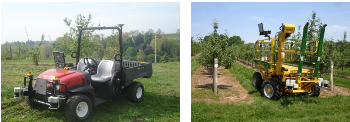
Figure 2. Examples of vehicles in the APM family. On the left is Laurel 1 , based on a Toro MDE eWorkman chassis. The two laser rangefinders on the front are used to find the tree rows closest to the vehicle. The information is passed on to the onboard laptop in front of the passenger seat; it finds the center of the row and guides the vehicle along it. Steering and wheel encoders complement the sensor suite and provide data for the computer to localize the vehicle along the row. On the right is Nittany, based on an Italian platform from N. Blosi. Because their sensing and computing architectures are the same, we are able to transfer row following and other autonomy software from one to the other with minimal or no rework.
