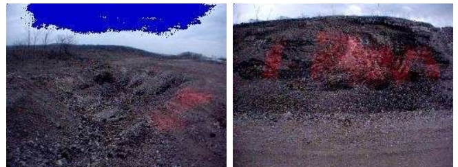
Fig. 12. Additional examples of novel instances identified during later traversal (red shade): first encounter with a ditch (left) and a large, heavily-sloped pile of rocks (right).
