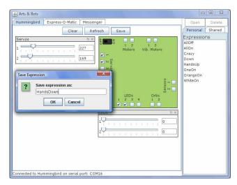
**Figure 1:** The programming software. Sliders are used to set the state of servos, LEDs, and other robot components. The set of state parameters are saved as an "expression" which can later be linked together with other expressions to form a simple sequential program.
