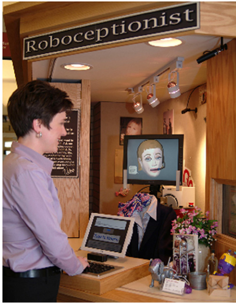
Fig. 2. A visitor interacting with Valerie, the Roboceptionist. The robot's virtual head is displayed on a monitor that rotates to face visitors. The robot's body—an RWI B21r—is "dressed" in a suit.
