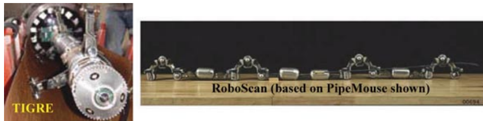
Figure 39. TIGRE and RoboScan: Additional prototype robot platforms under development for larger diameter unpiggable NG pipelines.
