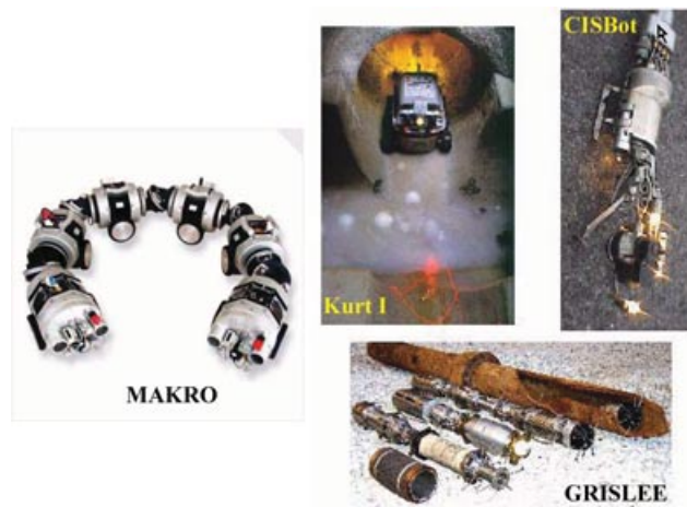
Figure 3. Representative tethered gasmain (CISBot and GRISLEE) and untethered autonomous (Kurt I and MAKRO) robots developed to date by industry/academia.
