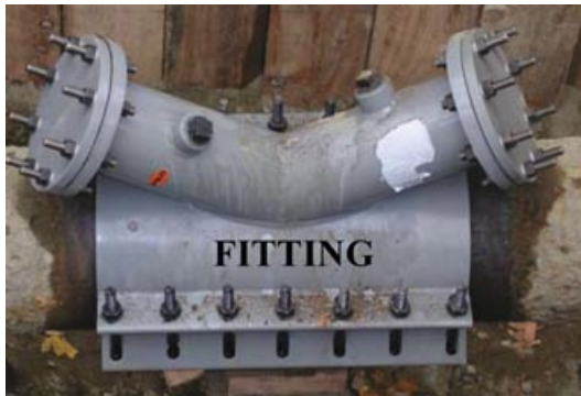
Figure 23. Low-pressure launcher fitting used for CI mains only.
