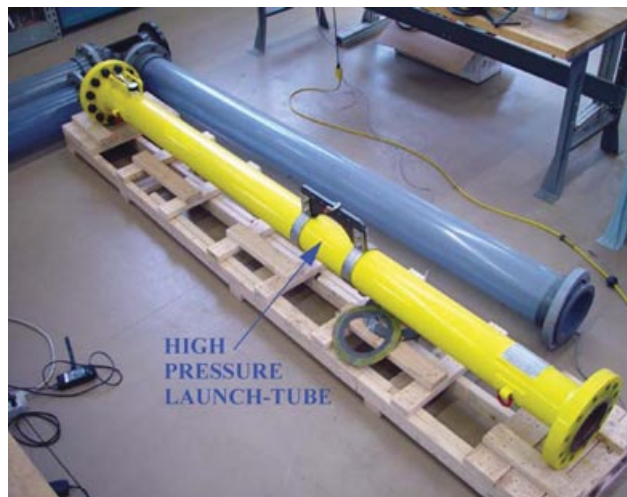
Figure 35. Launcher tube used for pressure testing to 750 psig for air and NG.
