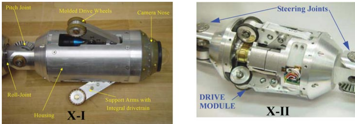
Figure 7. X-I (left) and X-II (right) drive-module design showing integral and removed camera nose.
