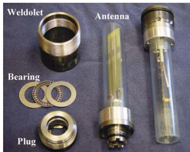
Figure 27. Antenna prototype as developed by ATK and adapted for use with Explorer.
