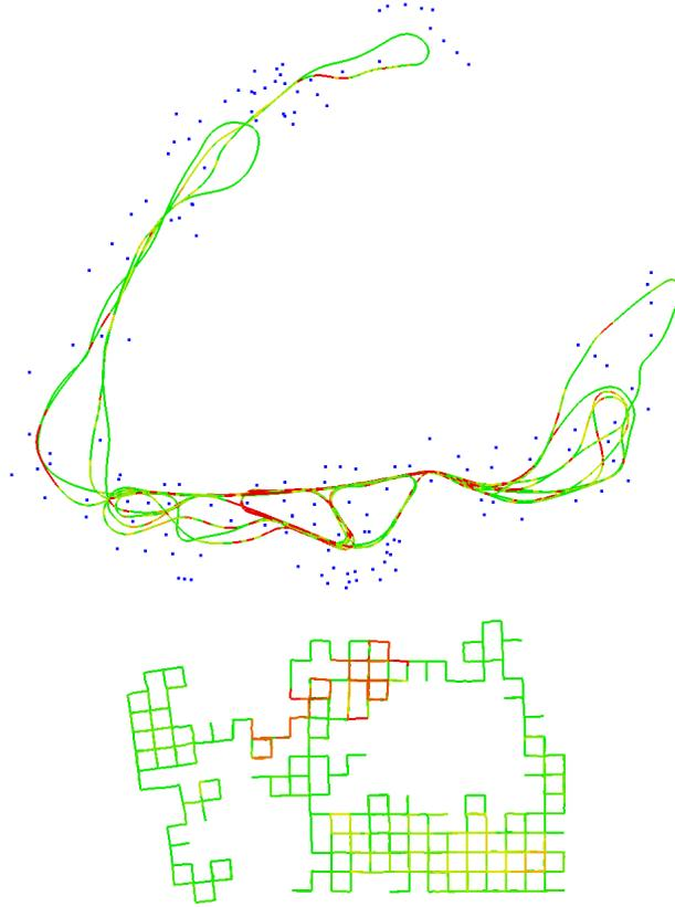
**Fig. 5** The Victoria Park dataset (top) and the simulated Manhattan world dataset (bottom) after optimization, color coded with the number of variables that are updated for every step along the trajectory. Green corresponds to a low number of variables, red to a high number.
