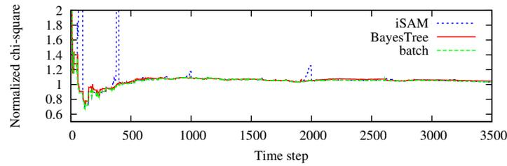
**Fig. 7** Comparison of normalized  $\chi^2$  for the simulated Manhattan world. iSAM shows some spikes where it deviates from the least squares solution because relinearization is only performed every 100 steps. The Bayes tree solution is always very close to the least squares solution because of the fluid relinearization ( $\beta = 0.05$ ).
