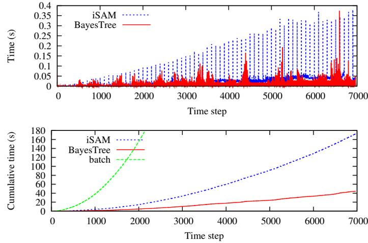
**Fig. 6** Timing comparison for the Victoria Park dataset. The top row shows per step timing and the bottom row shows the cumulative time. Our new algorithm (red) provides an improvement in speed over the original iSAM algorithm (blue), in addition to its advantages of eliminating periodic batch factorization and performing fluid relinearization. The original iSAM algorithm included a batch step every 100 iterations, which is clearly visible from the spikes.
