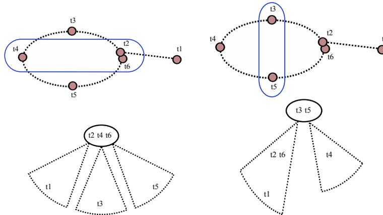
**Fig. 4** For a trajectory with loop closing, two different optimal variable orderings based on nested dissection are shown in the top row, with the corresponding Bayes tree structure in the bottom row. For the incremental setting the left choice is preferable, as the most recent variables end up in the root, minimizing work in future updates.
