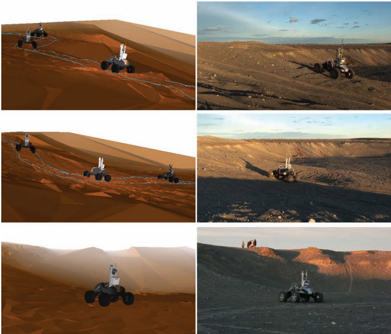
Fig. 19. Images of the terrain model with actual rover tracks, in cyan, overlaid (left) and photographs of Scarab while autonomously descending into a 9-m deep by approximately 100-m diameter sand pit (right). Terrain model constructed with triangular mesh in real-time for rover navigation and then re-rendered with atmosphere and light for an illustrative comparison.
