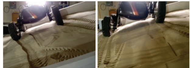
Fig. 13. Conventional posture normal to the slope (left) and actively controlled posture to maintain vertical (right) or to over-lean and edge wheels into the slope.
