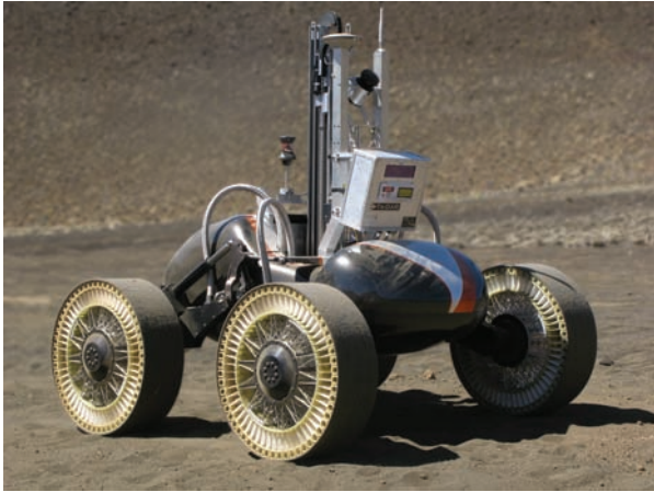
Fig. 6. Scarab rover with drill and instrument payload and Lunar wheels in fine basaltic soil at 3,000 m elevation on Mauna Kea in Hawaii.
