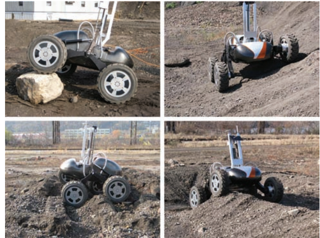
Fig. 5. Examples of climbing and suspension capability: surmounting a stable, wheel-diameter rock (upper left), active body-roll aiding in slope ascent (upper right), climbing offset obstacles (lower left), and egress from a rover-scale crater (lower right).
