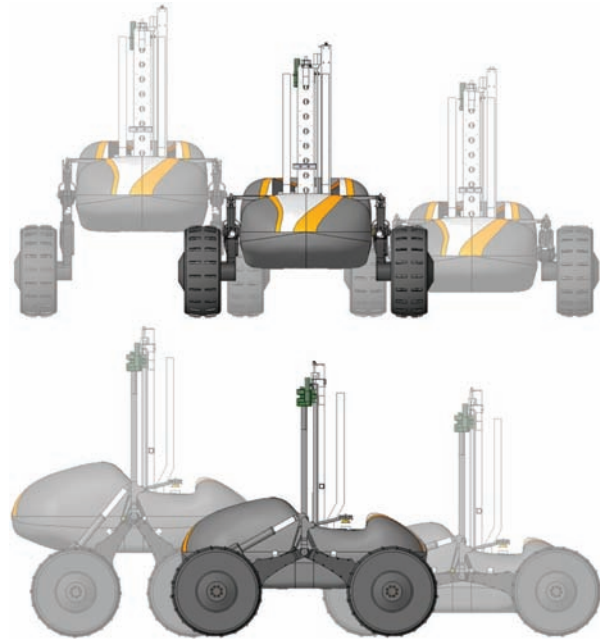
Fig. 4. Change to each side-frame angle, by adjustment of a linear actuator, changes the wheel base and ride height.
