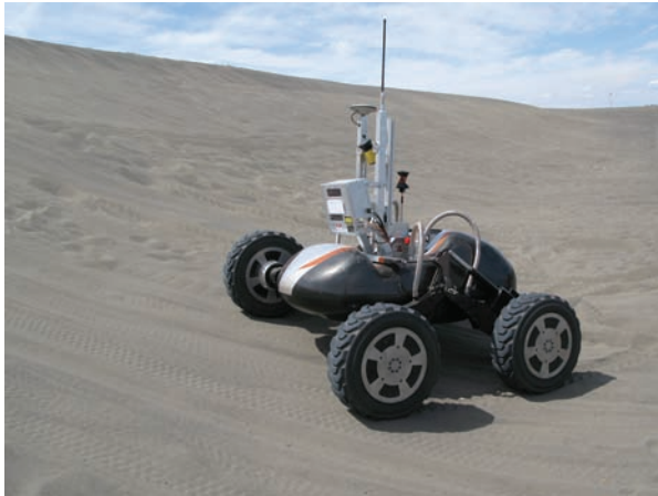
Fig. 1. Scarab Lunar rover prototype is designed to transport a coring drill and instrument payload while operating in the permanent darkness of polar craters. Shown in Moses Lake Dunes, WA.
