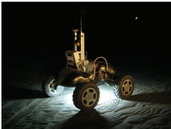
Fig. 16. Scarab navigating in darkness. The laser scanner perceives terrain ahead and an underbody optical velocity sensor estimates true velocity (without slip).
