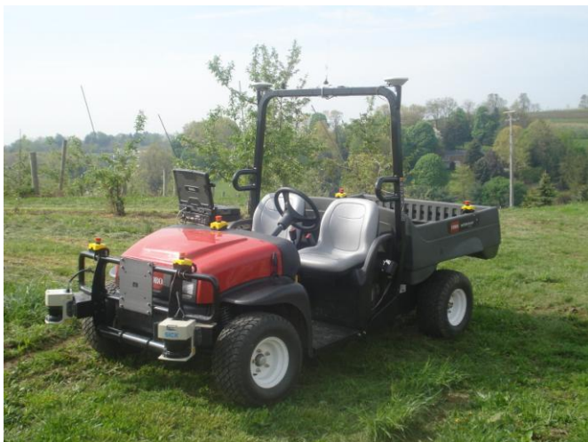
Figure 2. The Autonomous Prime Mover, based on a Toro Workman MDE utility vehicle.
