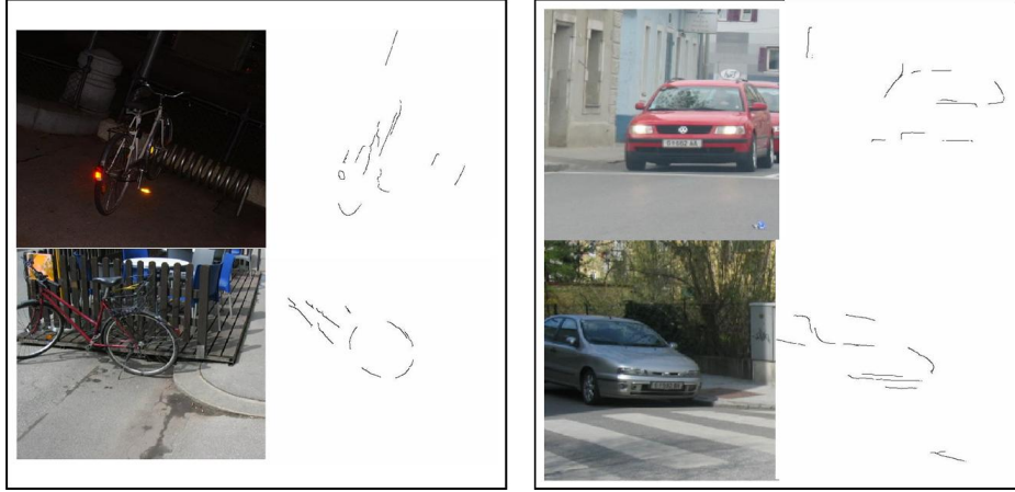
Figure 7.6: The model integrates geometric configurations belonging to different aspects (view-points) within the same category. Training images (left) and the boundary fragments containing the relevant parts learned from different view-points and integrated in the same model (right). Note that the algorithm automatically determines the features that belong to the object rather than the background.
