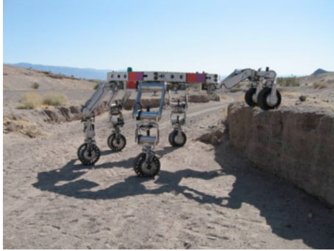
Figure 2.8: NASA’s ATHLETE robot has wheels on the ends of its 6 articulated legs for efficient rolling and stepping over obstacles [13].
