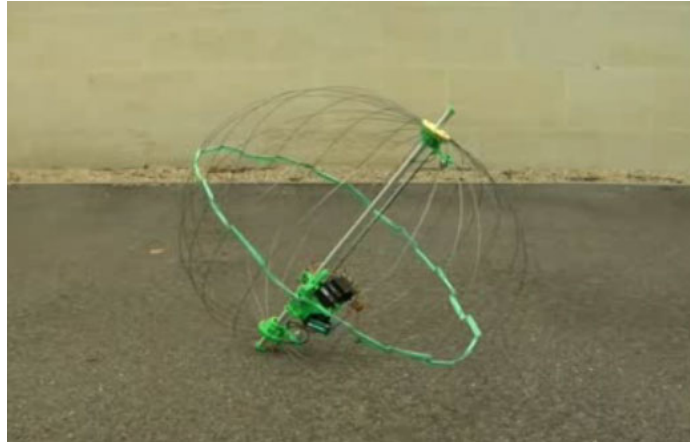
Figure 2.6: Jollbot from University of Bath elastically deforms its rolling cage to store energy for hopping [11].
