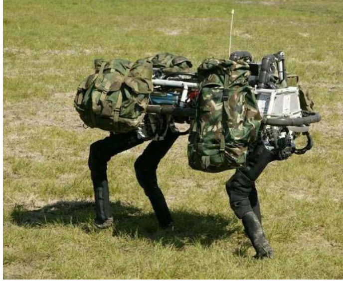
Figure 2.1: Boston Dynamics' BigDog is a legged robot that handles rough terrain by reactively maintaining its body posture [1].
