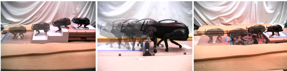
Figure 3: Multiple-exposure photos of LittleDog traversing various terrains from Phase II of the DARPA Learning Locomotion project. Left to right: steps, Jersey Barrier, and rocks.
