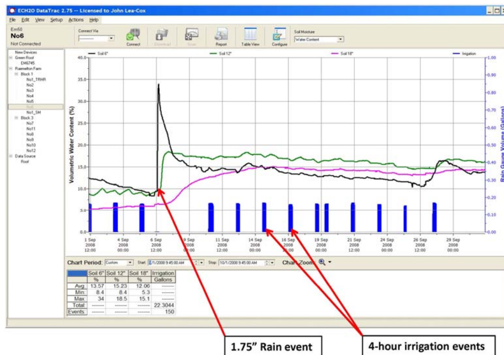
Fig. 4. A computer screenshot of the Decagon Devices, Inc. EchoTrac™ software, showing soil moisture data from EC-5 sensors at 6" (black), 12" (green) and 18" (purple) with rainfall and irrigation amounts from a sensor node in an Acer rubrum block in September, 2008.
