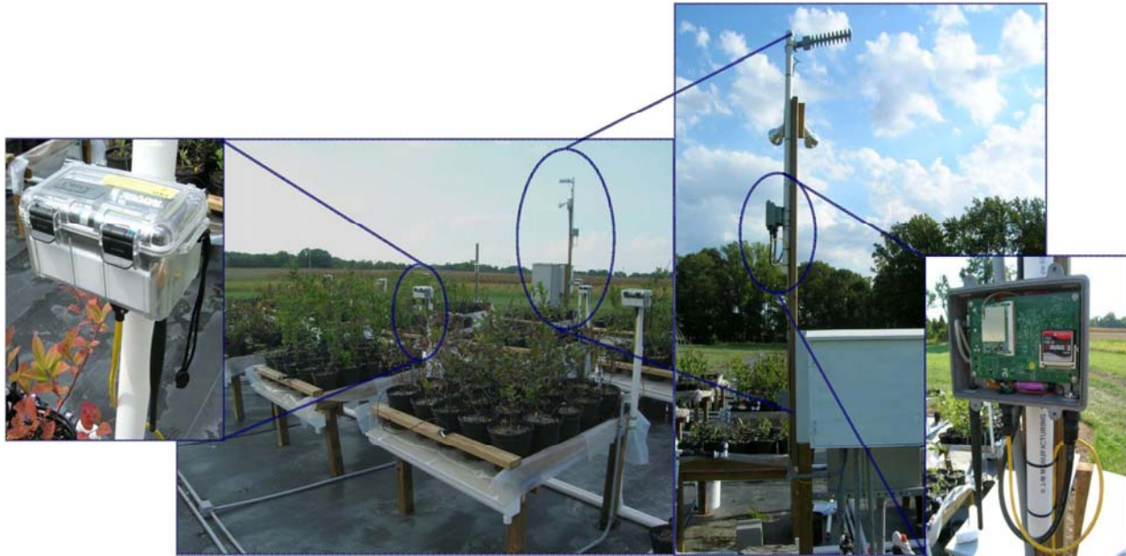
Fig. 2. The Carnegie Mellon University (CMU) network at the Wye Research and Education Center, near Queenstown, MD, showing sensor nodes (at left and centre), communication node and antenna (at right).
