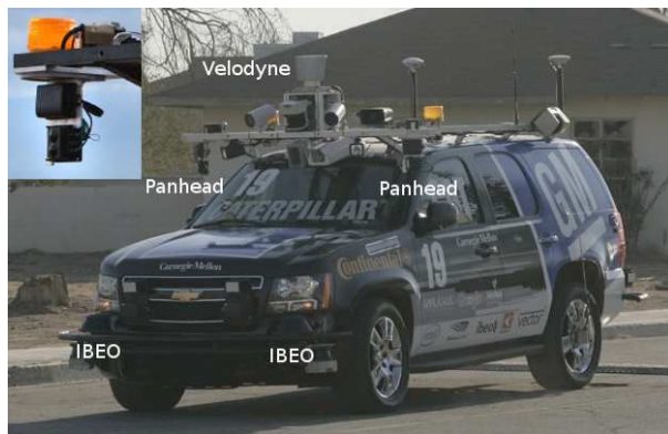
Fig. 1. The view of our robotic vehicle equipped with various sensors. Three different types of sensors are mainly discussed in this paper: A Velodyne HDL-64 at the top, two IBEO Alasca XT on both sides of the hood, and two ARS-300 installed on the panhead platforms on the driver and passenger side.
