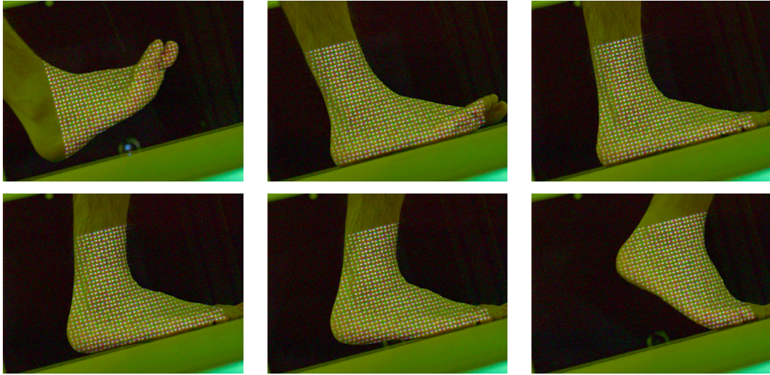
Figure 11: Input images for the foot side measurement. The subject is walking.
