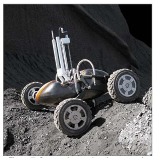
Figure 7: Suspension conforming to terrain
