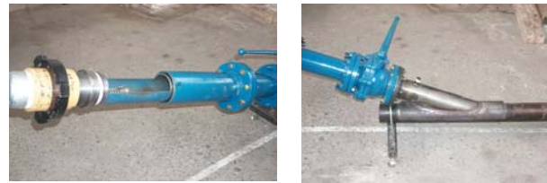
Figure 10 : Live gasmain access and launch fitting
