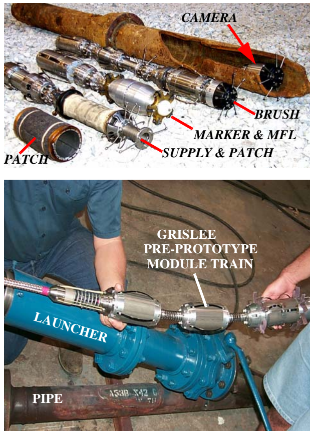
Figure 12 : Train-configurations and pre-prototype test-launch experiment
